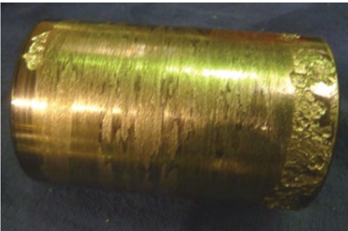
Bearing rollers showing pitting and spalling damage.
