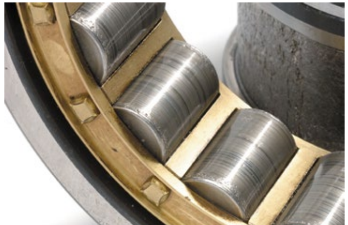
Bearing rollers showing pitting and spalling damage.
