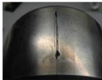
Fig. 1 A single axial crack that has propagated completely through the inner ring.
