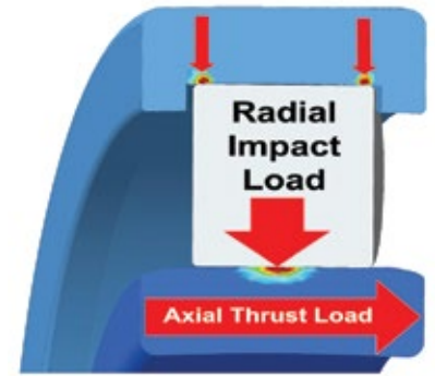
Fig. 9 – Image showing the simultaneous radial impact and axial loading of the misaligned roller.
